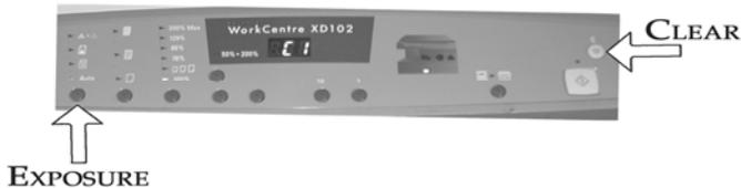
Enter the diagnostics menu by turning the machine on, and within 4 seconds, press "CLEAR", "EXPOSURE MODE", "CLEAR", "EXPOSURE MODE". (EXPOSURE MODE is the button on the far left). All of the display will go blank. Using the 10 and 1 buttons (copy quantity), enter "24" press "PRINT", enter "7" press "PRINT" again. The counter is now set to Zero!
