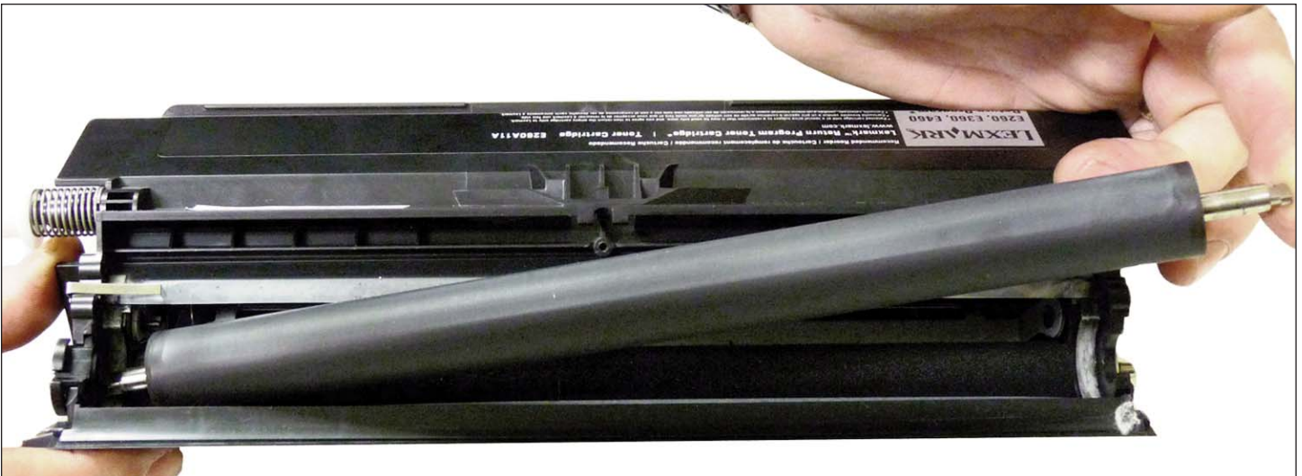
12. Remove the developer roller. Clean the toner feed roller with compressed air.
