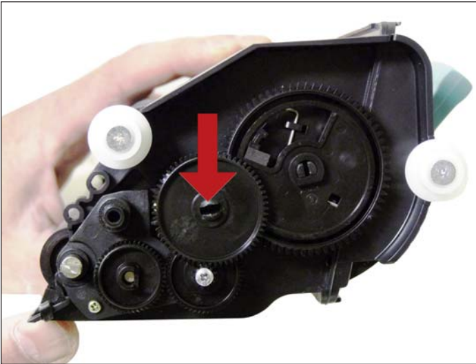
8. Remove the large idler gear by pressing in the 2 clips in the center of the gear.
