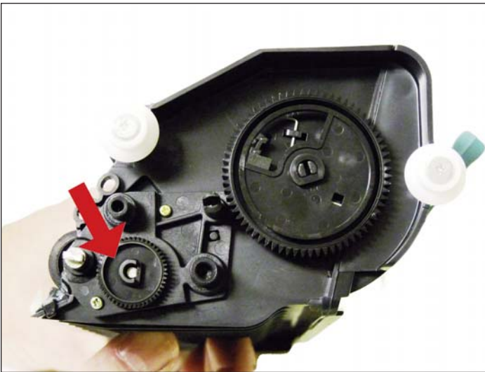
10. Remove the feed roller gear. This has a tight fit. Pry off carefully.
