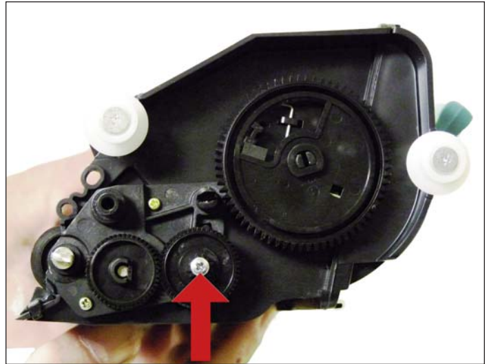
9. Remove the screw and lower idler gear.
