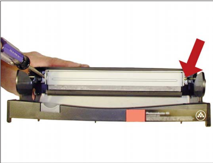
8. Install a new wiper blade coated with your preferred lubricant and two screws.
