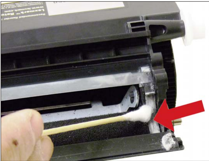
13. Clean the white developer roller seals with a cotton swab.
