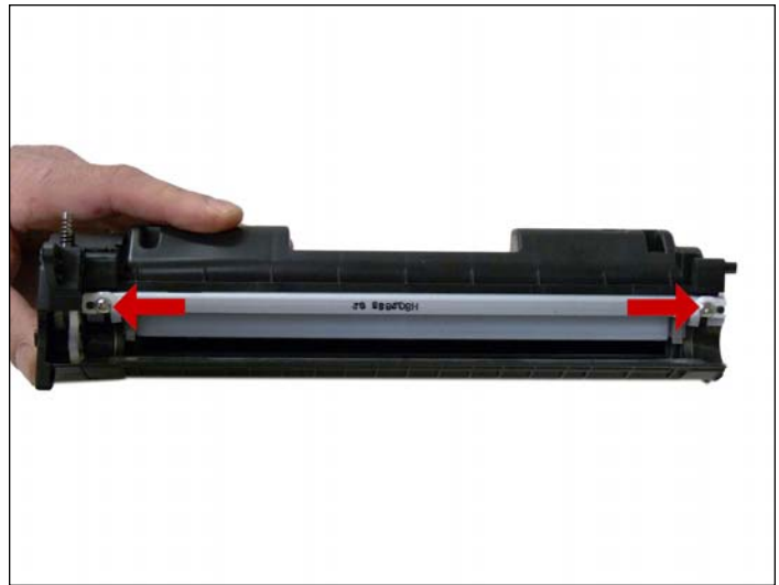
17. Remove the doctor blade and two screws.
