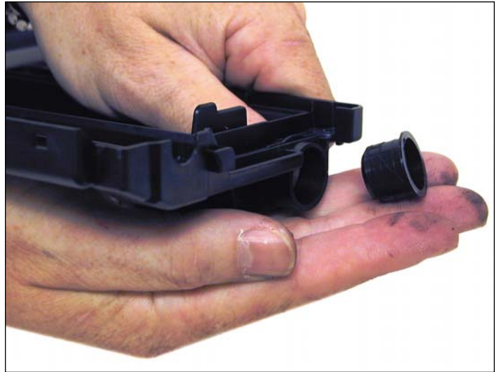
19. Remove the fill plug from the top cover.
