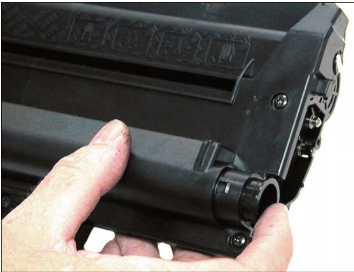
24. Install the fill plug, check for leaks.
