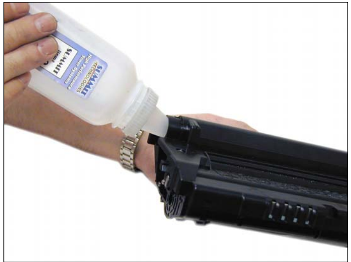
23. Fill the hopper with the SCX-4300 toner.
