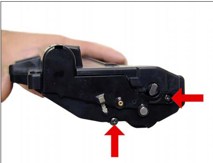
25. Install the remaining end cap and two screws. Make sure the top of then end cap snaps into place over the fill plug
