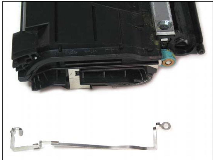
14. Remove the doctor blade contact which runs along the side of the cartridge.
