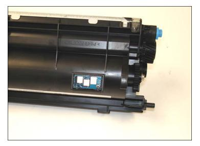
16. Install the UniNet chip and place again the little screw. Finally, install the develop roller cover for shipping.
