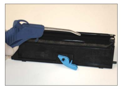
8. Use compressed air to clean residual toner from the toner hopper section. Place the foam properly as a bad installation would cause leaking.
