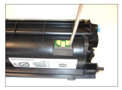
14. Use a screw driver to remove the small screw that secures the chip.
