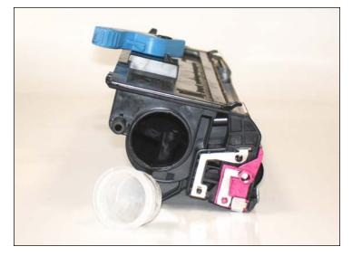
1. Remove the hopper fill plug and dump the remaining toner with compressed air. We don't recommend using a vacuum cleaner with a plastic nozzle or a non earth compressed air device since it could generate electrostatic charges.
