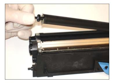
4. Take out the develop roller by its left part reminding the position of the sealing mylars on each extreme of the roller.
