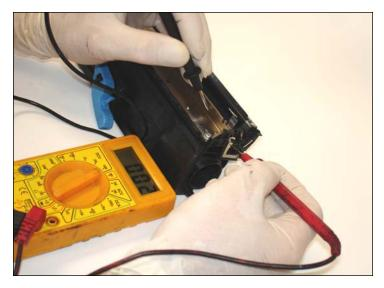
12. Check the electrical continuity with a tester to ensure good contact between the doctor blade and the main contact.
