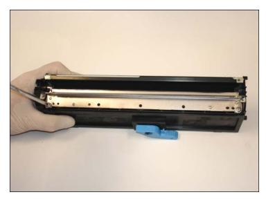
6. Remove the two screws that fix the doctor blade.
