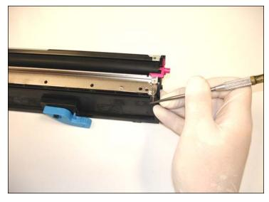
2. Release both springs on each extreme of the doctor blade using a spring hook tool. Use a small screw driver to remove the pink plastic develop roller stabilizer, too.
