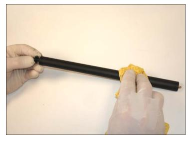
10. Clean the develop roller with compressed air. Afterwards use a lint-free cotton pad with distillate water (70%) and isopropyl alcohol (30%).
