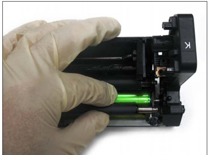
19. While removing the large end cap hold the PCR as it will tumble off when the end cap is being removed. Once you free the PCR remove it, then continue removing the end cap.
