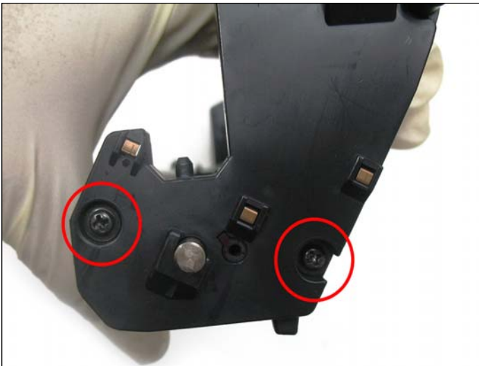
18. Remove the larger end cap first by removing the two screws as shown.
