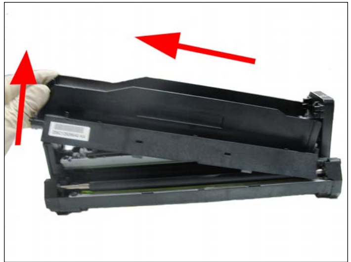
14. Remove the top cover by first lifting the left side and pulling away from the cartridge as shown.
