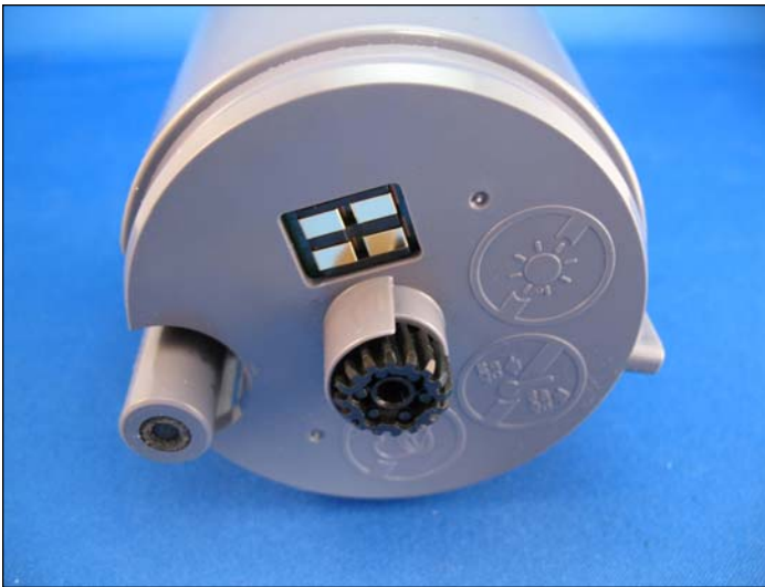
3. Gear side of cartridge with OEM chip.
