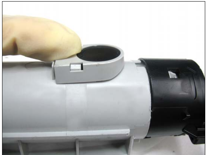
29. Press down until the tabs lock it into place.
