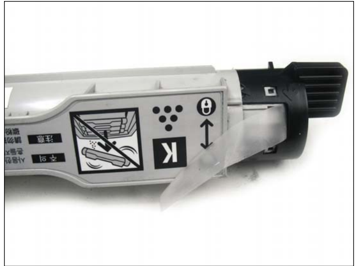
21. Push the end cap inward until it latches onto the four locking tab mechanisms. Make sure all four tabs are properly secured.
