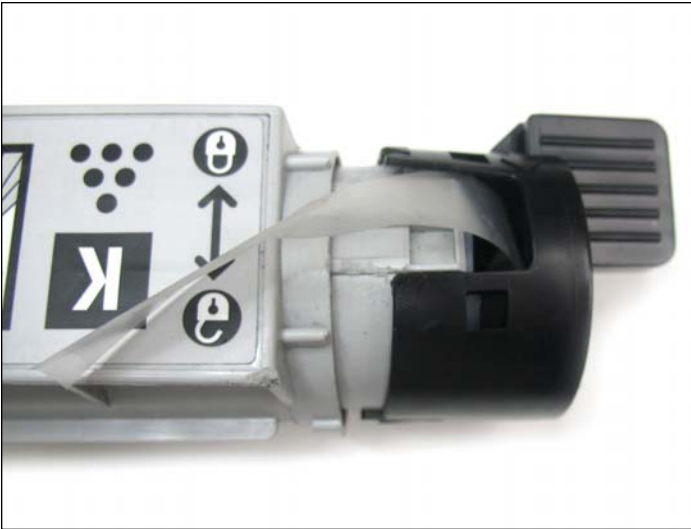
20. Place the gearless end cap, in its original positioning, over the seal and toner fill plug as shown.
