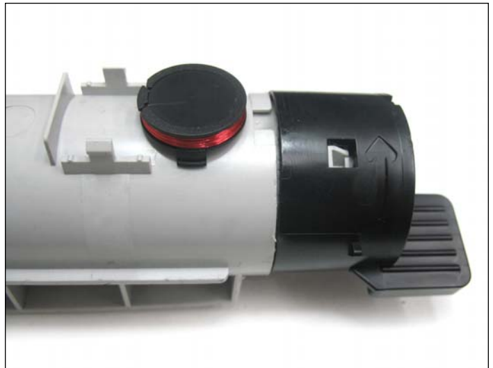
27. Place the new contact chip on the cartridge in the manner shown.
