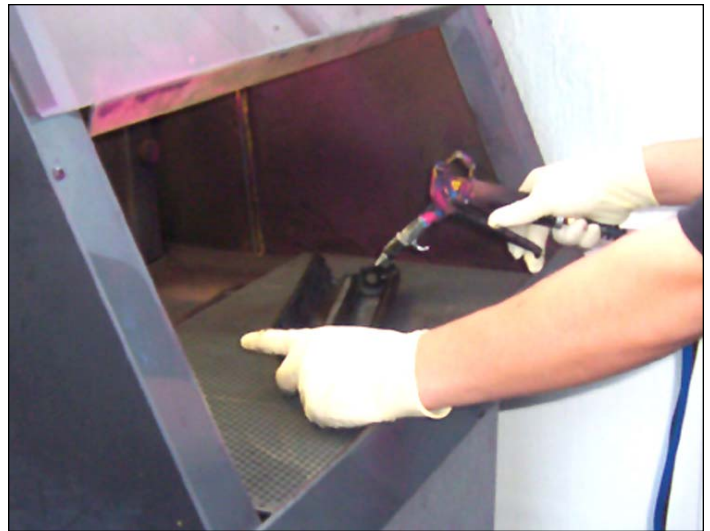
24. Clean using air pressure. Reassemble when done.
