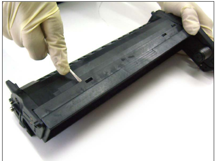
4. Turn the plastic cover upside down and pry open the back side with a small flathead screwdriver as shown.
