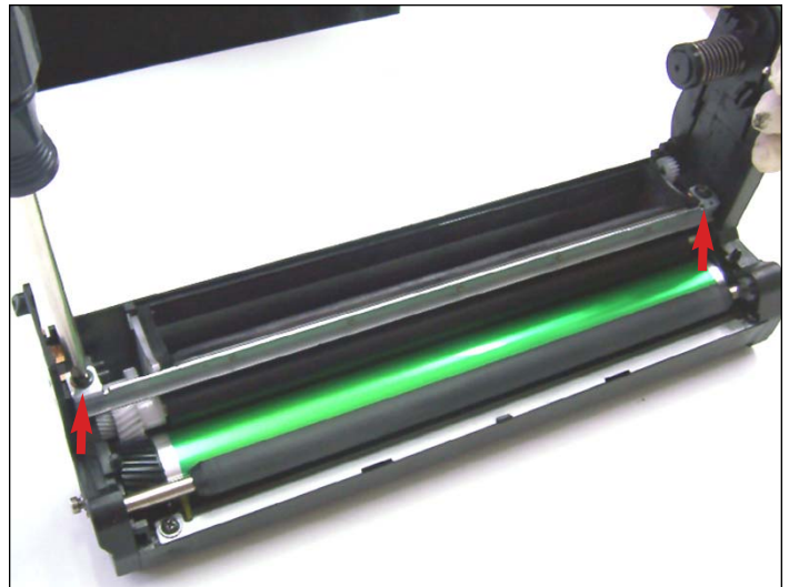
8. Remove the two screws from the ends of the Doctor Blade that is connected to the end caps.
