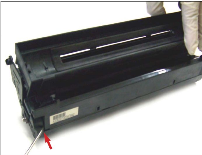
5. Turn it right-side up again and pry open the front side as shown.
