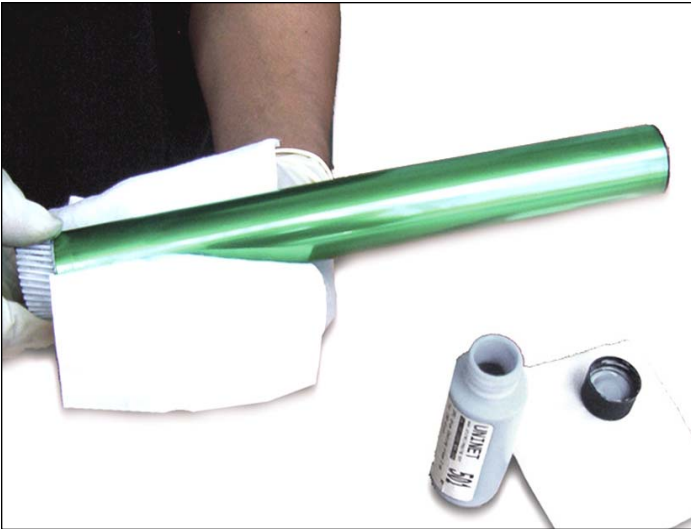
19. Apply UNINET "OPC Drum Coating Cream" #501 to preserve the life of the cylinder.
