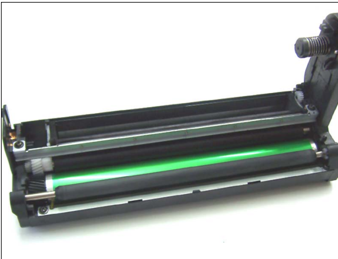
7. You are now ready to disassemble the drum unit.
