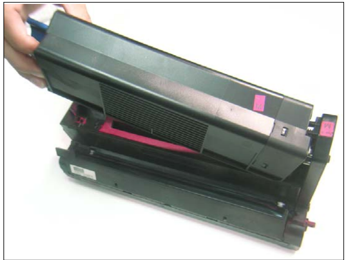
2. Remove toner unit and set aside.
