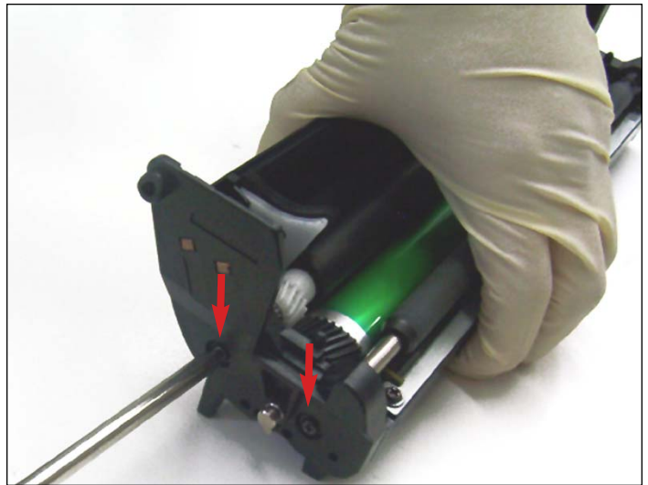
10. Remove the two screws located on the side of small end cap as shown.
