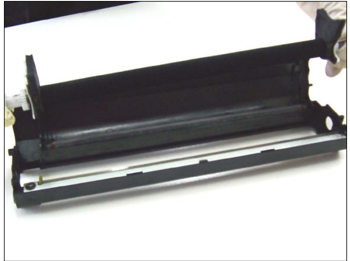
20. Remove the supply roller and its components as shown.
