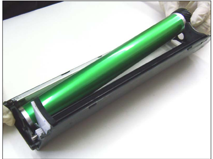
18. Carefully remove the cylinder as shown gear-side first.
