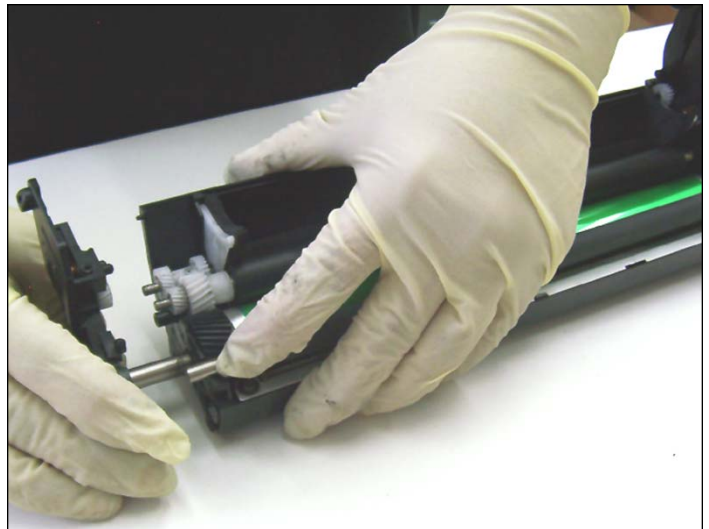
12. Once you have removed the screws, pull the small end cap out.
