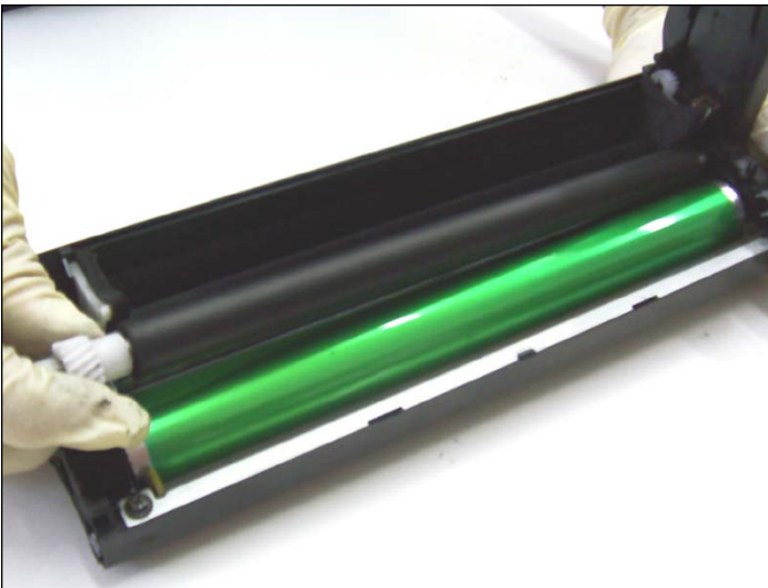
15. The developer roller should come out easily.
